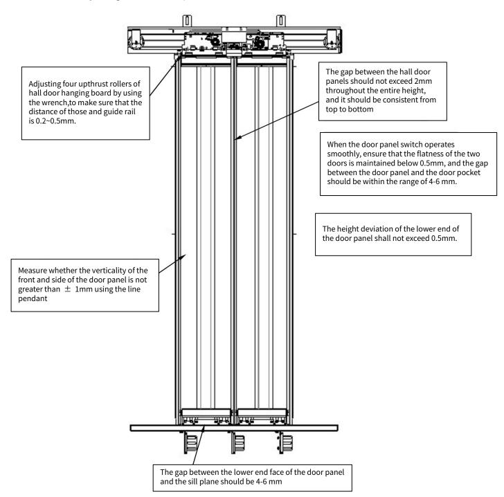
Open hall door to the position and make one hall door is on an even height with jamb , check if the other hall door is on an even height with jamb . If there is a deviation, it indicates that there is a deviation between the center of hall door and the center of door jamb . It needs to be readjusted, generally by adjusting the Interlocking steel sire rope connecting the two hall door , and adjusting its left and right position fixed on the hanging board.
