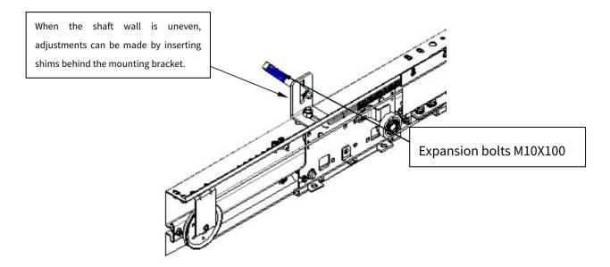
4. Install expansion bolts at the corresponding positions of each fixed foot of the door pocket on the shaft wall to prepare for fixing the jamb.
