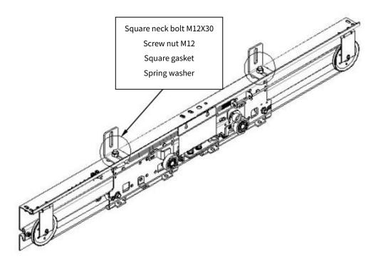
2、Preset the header and connect the header to the jamb header bracket.
