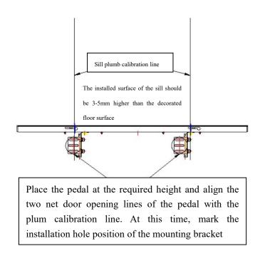
4. Remove the sill and brackets at both ends, drill holes on the marks with an impact drill, and
