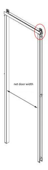
2. Fix the lower end of Jamb to the sill with bolts
