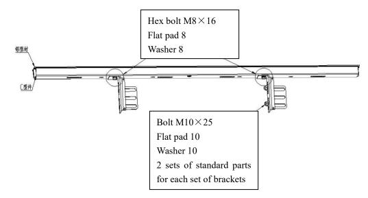
3.Determine the position of the mounting holes for the brackets at both ends and make a mark at this position. As shown in the following figure
