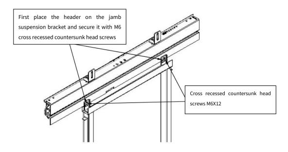
3. Determine the position of the header installation bracket, align the net opening scale lines on both ends of the header with the door sample line, and then install expansion bolts to secure the header.Installation and adjustment of hanging panels and door panels
